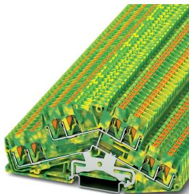
Double-level terminal block, number of connections: 8, connection method: Push-in connection, 1st and 2nd level, Rated cross section: 2.5 mm<sup>2</sup>, cross section: 0.14 mm<sup>2</sup> - 4 mm<sup>2</sup>, mounting type: NS 35/7,5, NS 35/15, color: green-yellow
